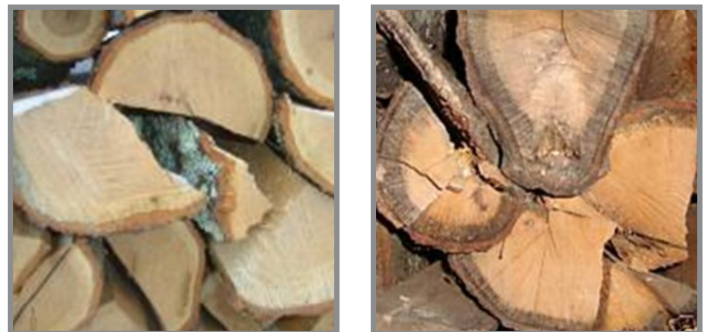
Figure 1. Fresh cut oak wood on left and dried oak on right with wood splitting at ends and discoloration.
