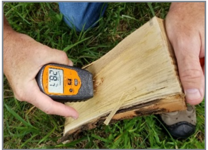
Figure 3. Proper moisture measurement involves splitting a piece of wood and taking measurement in the middle of log. 20% is best. Higher readings will require more drying time.
