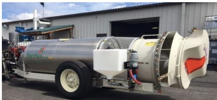
Fig 1). Harvista™ application using a standard commercial applicator fitted with an AgroFresh formulation tank, seen as the large white container, accompanied by the Injection pump to the right of the formulation tank. Source: AgroFresh.
