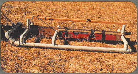
EM-38 being used on a PVC sled near Valley City, N.D.
