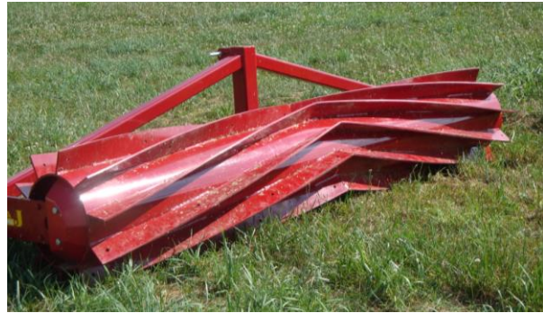
Figure 9. Roller/crimper used to create dead-mulch layer
