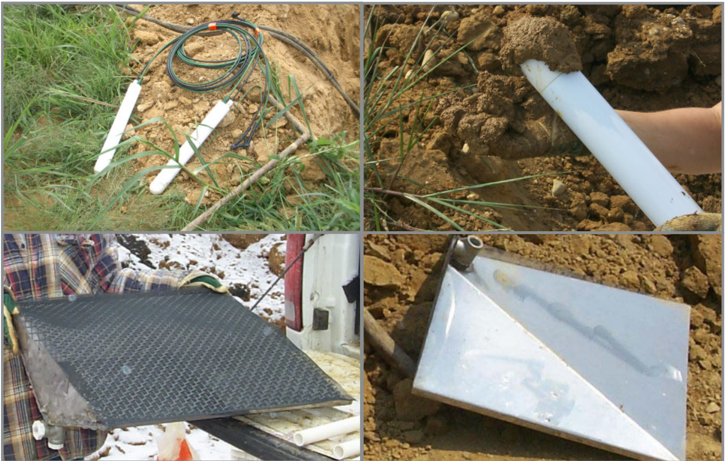
Figure 17. (top left) Suction lysimeters are a PVC tube with a porous ceramic tip that is kept under suction to sample soil water. The plastic line allows the collected water sample to be extracted from the surface and suction then reapplied to collect another sample. (top right) A mud made of native soil is put on the ceramic cup during installation to insure good contact and moisture movement. (bottom left) Pan lysimeters constructed of stainless steel capture vertical flow. Surface screening on the pan stops soil from entering the pan. (bottom right) The bottom of the lysimeter is in a shape that allows good contact with soil above it during installation and will retain approximately 7 liters. The lower part of the collection pan is connected via a plastic line to the surface and allows the extraction of the sample water on a regular basis.
