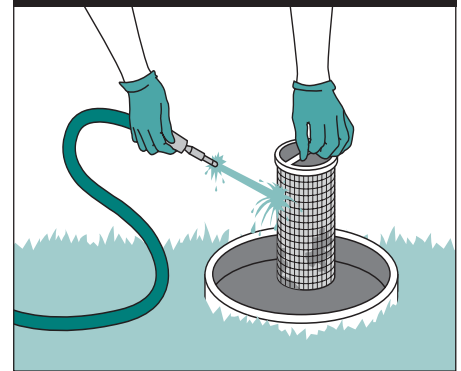
FIGURE 7.17 Cleaning an Effluent Screen
