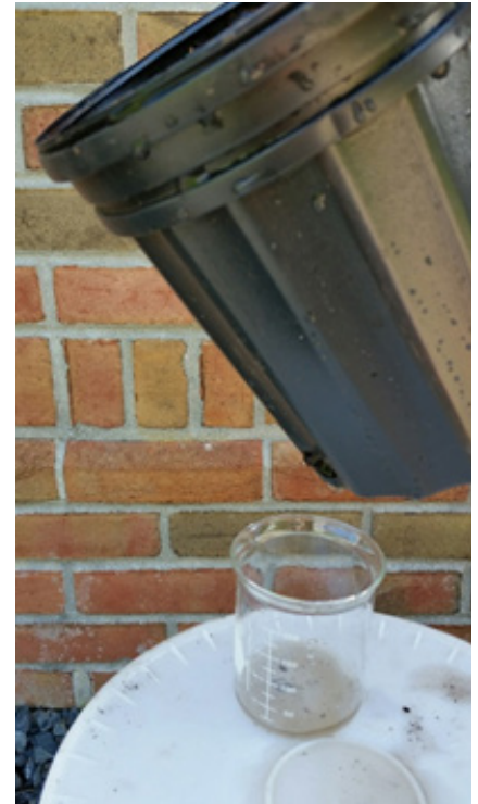
Tipping pot after an irrigation event to gather a water sample Photo: Andrew Ristvey, UME
