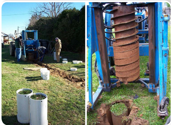
Fig. 1. Tractor-mounted soil corer was used to collect undisturbed lysimeters (12 inches diameter and 20 inches deep).
