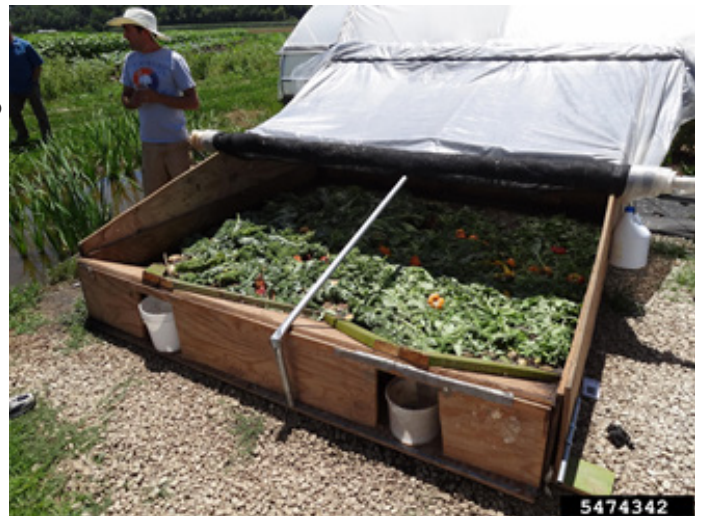
Biocomposter for raising soldier flies to produce fuel from the pupa. Photo: J. LaForest, UGA, Bugwood.org
