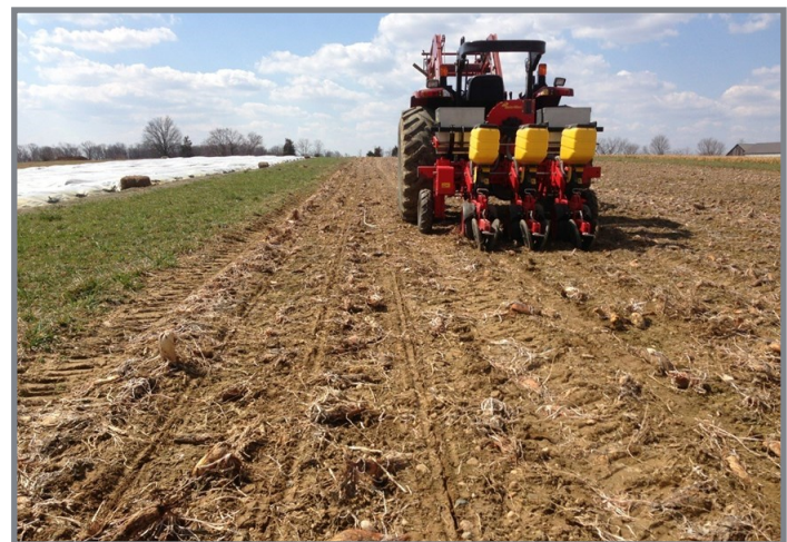
Figure 12: Heavy seeders with coulters and/or double disk openers have no trouble slicing through radish residue. Adjustments may be necessary for adequate furrow closing. Photo: Dave Liker.
