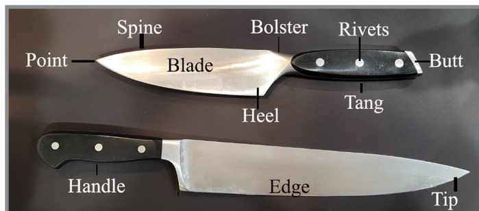
Figure 2.1: Basic parts of a chef's knife. Most knives have these features. Photo by S. Henley
