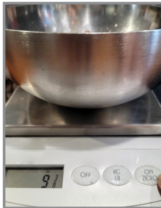
Figure 3.8: Using the Zero or Tare button will remove the weight of the container from the scale’s measurements. Photo by S. Henley
