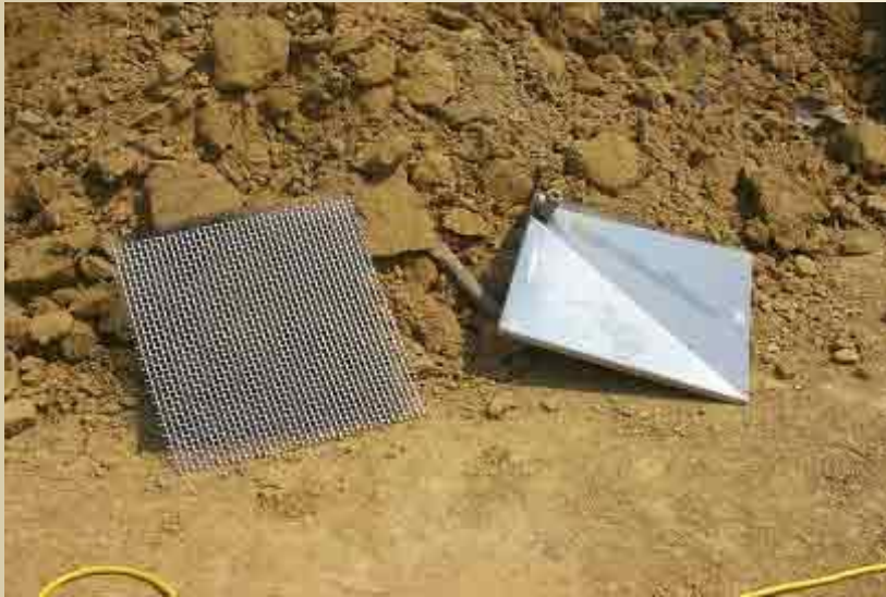
Lysimeter pan inserted below filled trench with access tube
