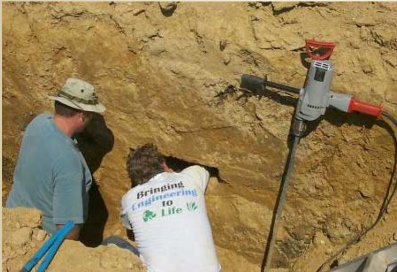
Lysimeter pan inserted below filled trench with access tube
